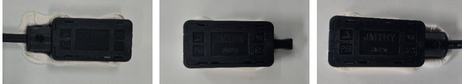
Fig. 3: View of junction box of module type ERA Pro-72HC585M
